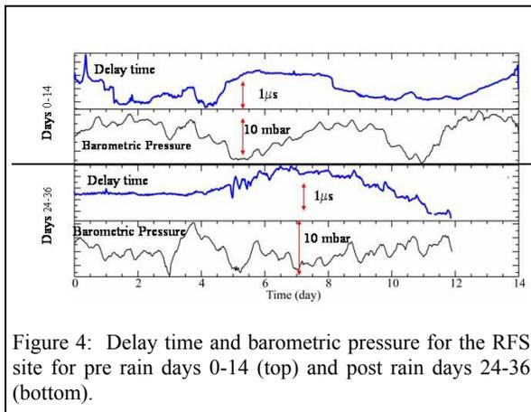
Figure 4: Delay time and barometric pressure for the RFS site for pre rain days 0-14 (top) and post rain days 24-36 (bottom).
